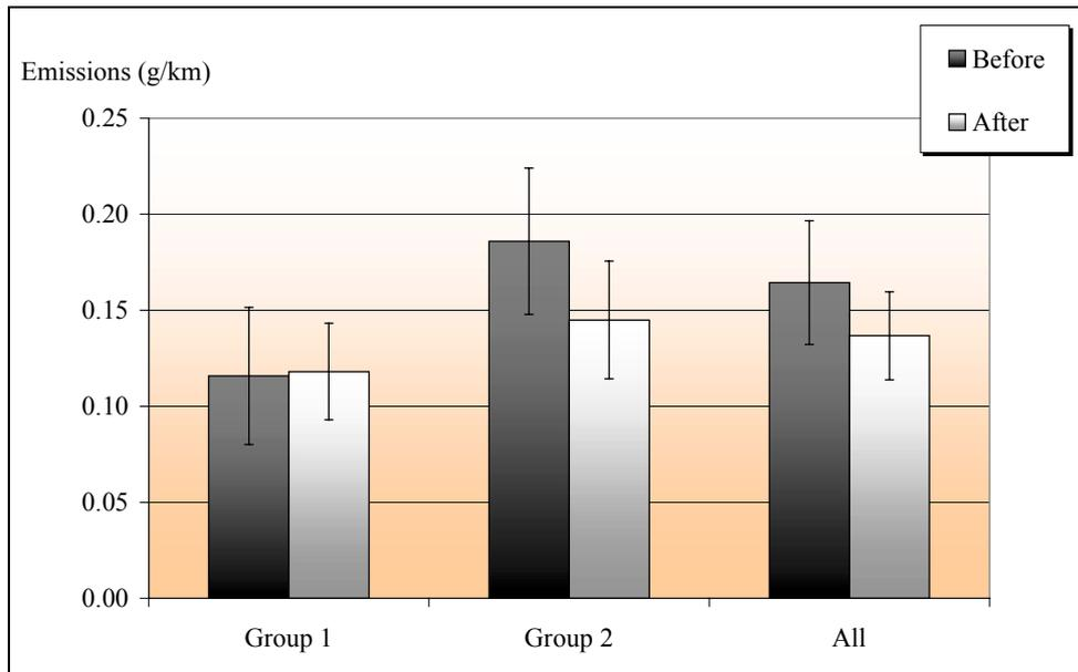
Figure 4.17 Emission of nitrogen oxides before and after instruction for the two groups and the average for all the students. The lines mark the limits for 95 per cent confidence intervals for the average value.
