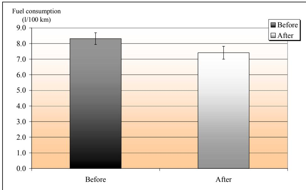
Figure 3.8 Fuel consumption before and after instruction. The line indicates the limits for the average value, including a 95 per cent confidence interval.
