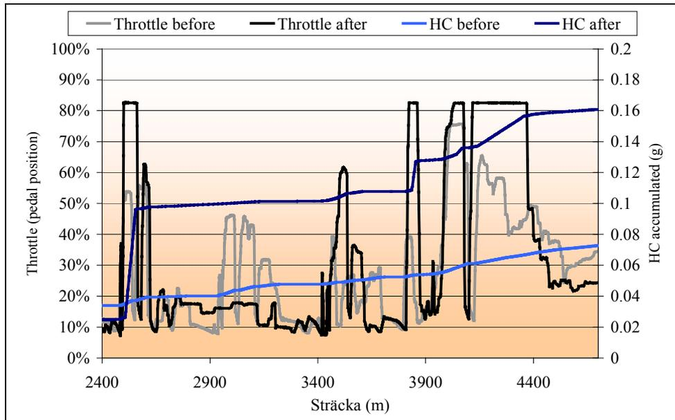
Figure 4.6 Throttle and emissions of hydrocarbons for the driving patterns in Figure 4.4.
