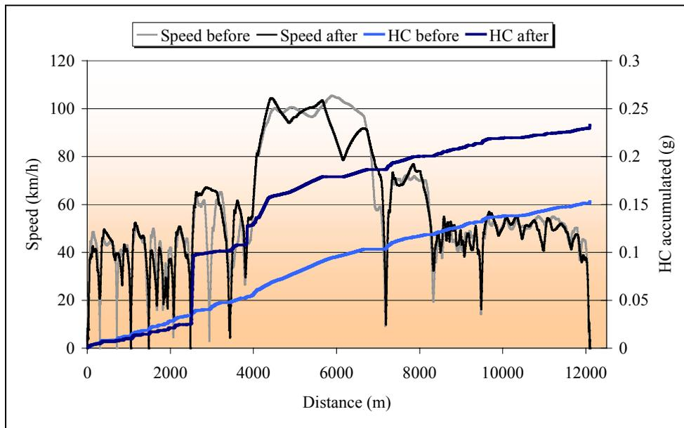
Figure 4.3 Driving pattern and emissions of hydrocarbons for a student in Köping before and after instruction.
