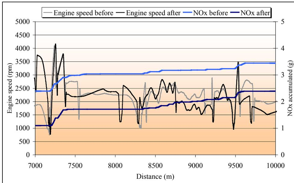
Figure 4.12 Engine speeds and emissions of nitrogen oxides for the driving patterns in Figure 4.11.
