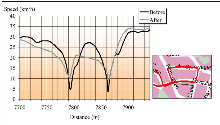
Figure 3.3 Comparison of driving styles before and after training in EcoDriving in Solna. The first minimum speed took place when the driver braked before the intersection between Björkvägen and Filmgatan. The driver then turned 90 degrees and increased speed before braking, after which a new minimum speed took place before the intersection between Filmgatan and Lövgatan.
