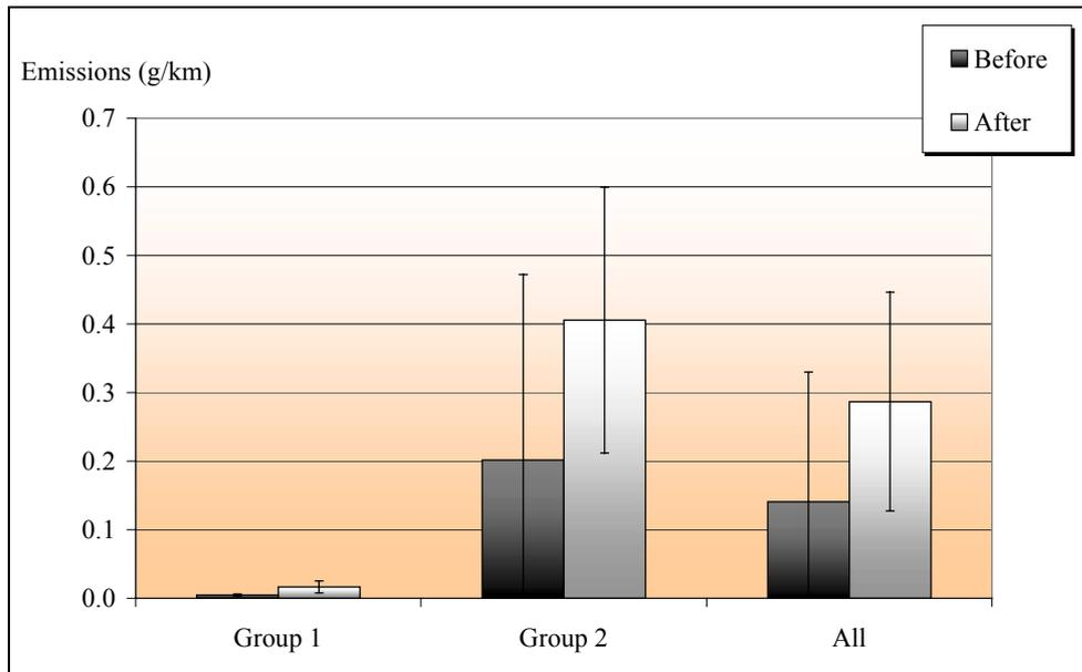
*Figure 4.15* Emission of carbon monoxide before and after instruction for the two groups and the average for all the students. The lines mark the limits for 95 per cent confidence intervals for the average value.
