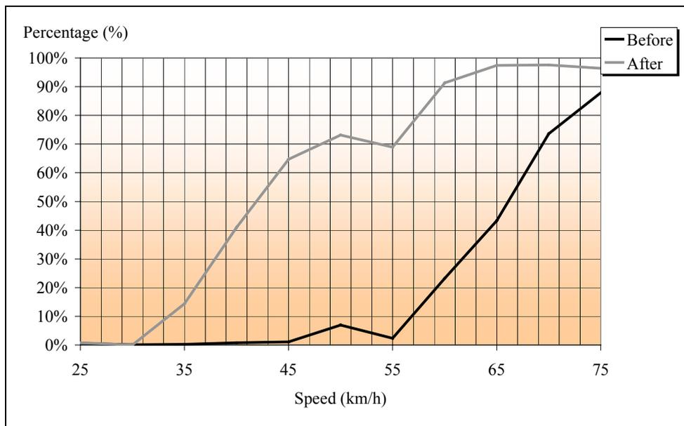
Figure 3.6 Percentage of driving in fifth gear at constant speed.
