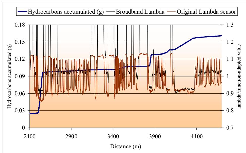
*Figure 4.18* Comparison of a broadband Lambda sensor (Rototest IVAS) and an original Lambda sensor. To facilitate the comparison, the value from the original Lambda sensor has been adapted according to  $(-1(\text{original} + 0.85))$ .
