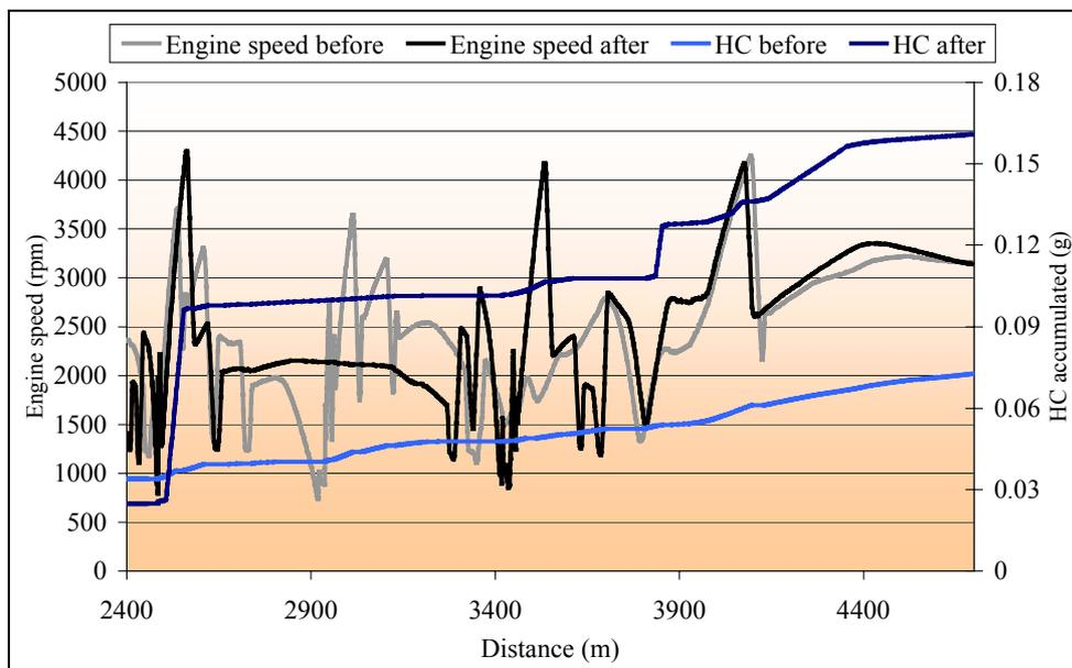
Figure 4.5 Engine speeds and emissions of hydrocarbons for the driving patterns in Figure 4.4.
