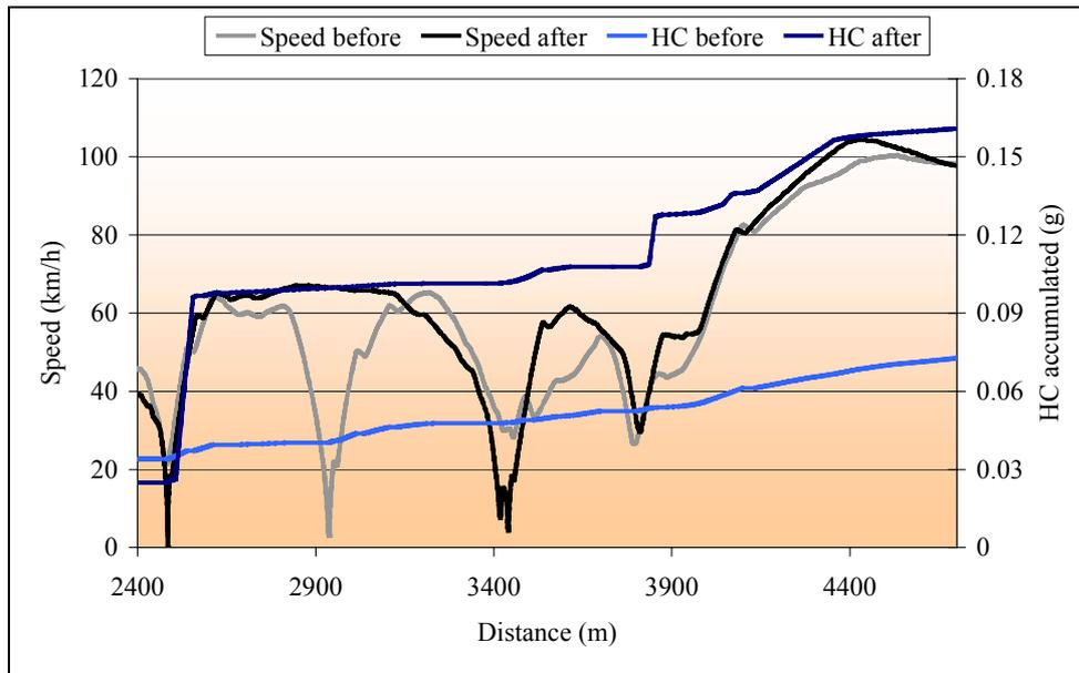
Figure 4.4 Details of driving pattern and emissions of hydrocarbons for a student in Köping before and after instruction.
