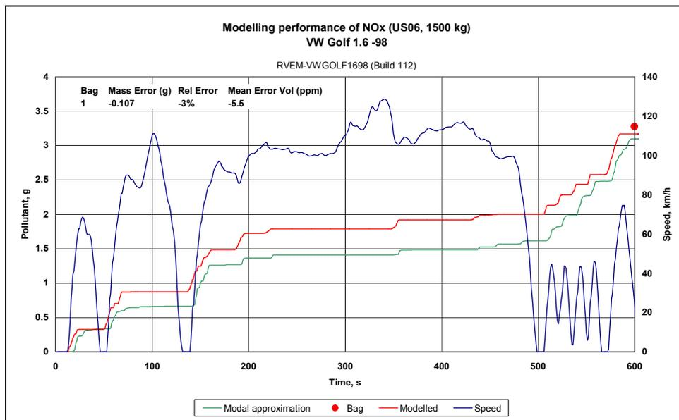
Figure 2.4 Example of an evaluation of a model for a 1998 VW Golf 1.6.
