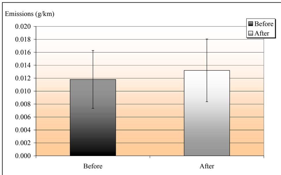
Figure 3.10 Emission of hydrocarbons before and after instruction. The line indicates the limits for the average value, including a 95 per cent confidence interval.
