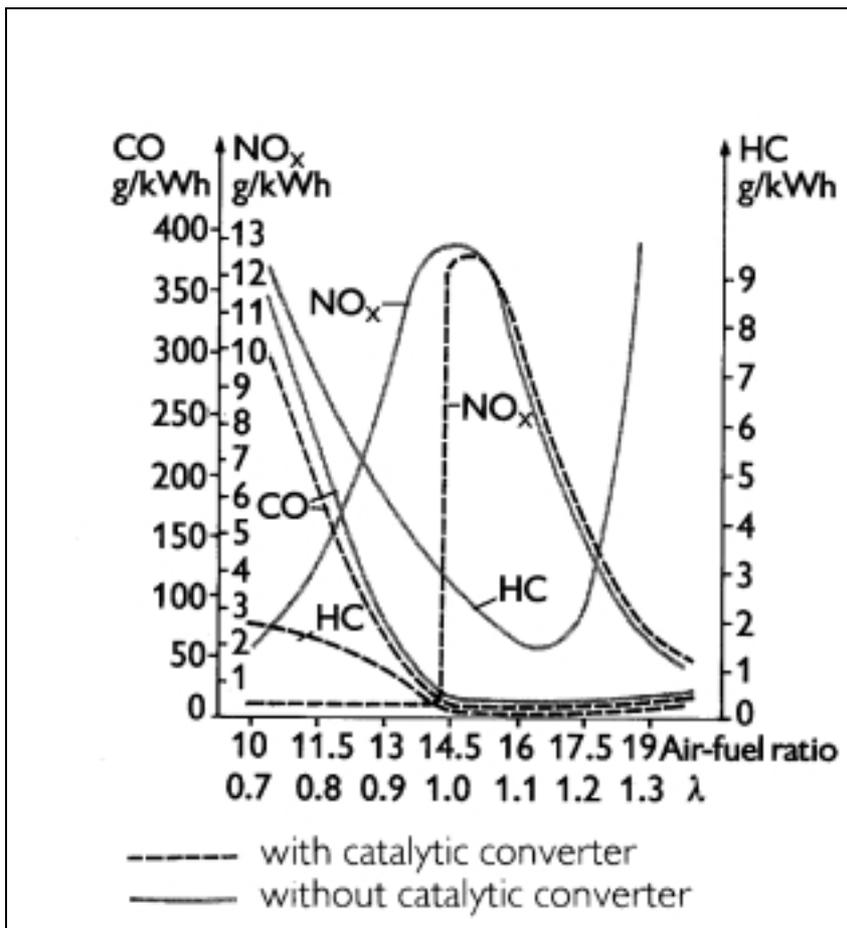
Figure 4.1 Emission control using a three-way catalytic converter (Bauman, 1988).
