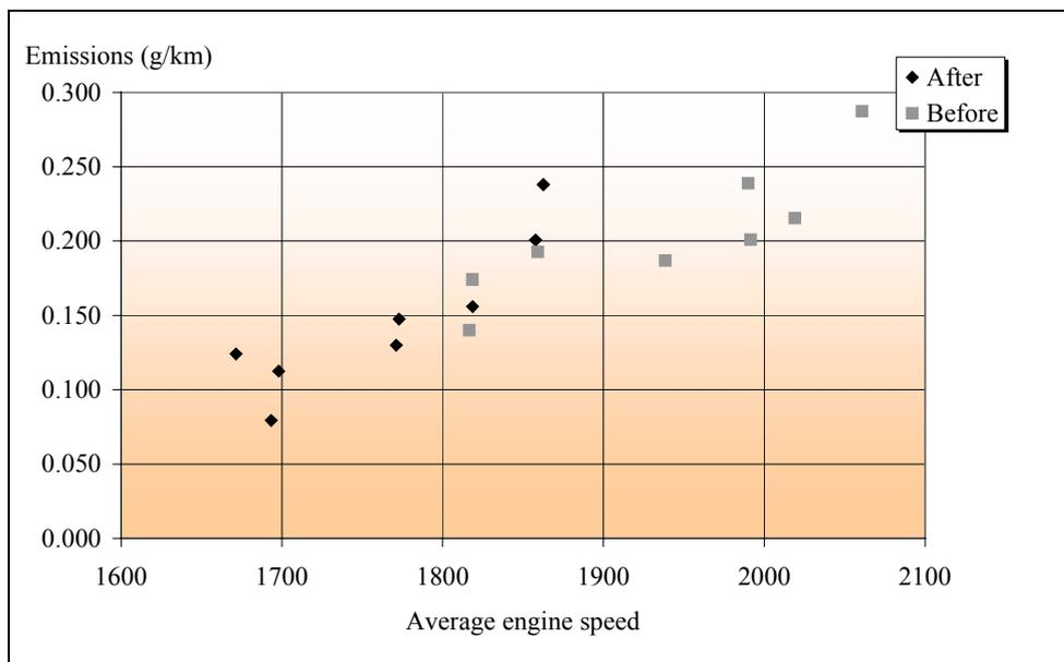
Figure 4.13 Relationship between emission of nitrogen oxides and average engine speed for the journeys before and after instruction in Köping.
