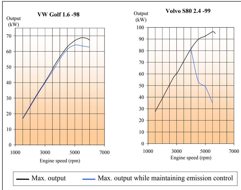
Figure 4.2 Maximum performance while maintaining emission control for a 1998 VW Golf 1.6 and a 1998 Volvo S80 2.4. The figure shows how much output can be obtained at different engine speeds in static conditions while maintaining full emission control, compared with the maximum output obtained at the corresponding engine speed. N.B. Different scales (source Rototest AB).
