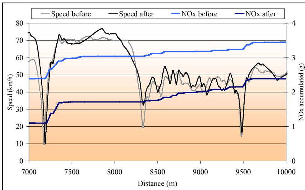
Figure 4.11 Details of driving pattern and emissions of nitrogen oxides in Figure 4.10.
