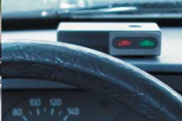
A new type of informative ISA system was tested in Borlänge and Lidköping where the driver was informed about the prevailing speed limit via a display. If he or she drove too fast, a sound signal was heard and a light turned on. This system knows the speed limit through an onboard computer that compares the co-ordinates from the GPS receiver with a digital map onto which the speed limits have been entered.
