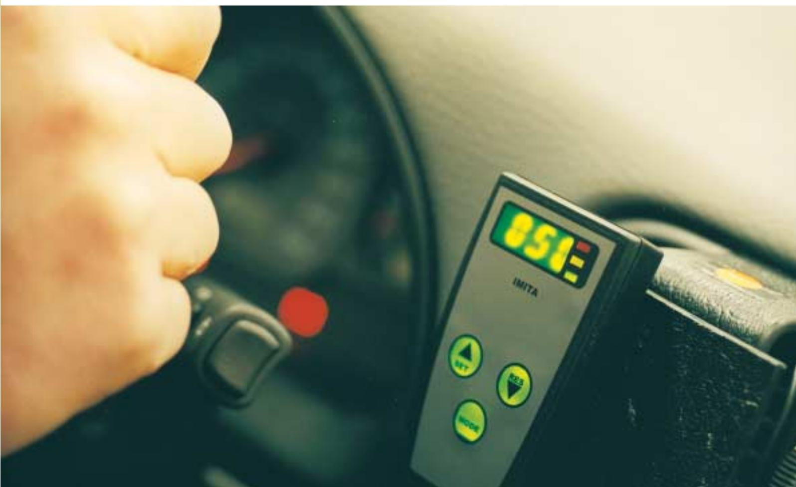
A supportive ISA system was tested in Lund and Lidköping where the driver received information about the prevailing speed limit via a display. If he or she drove too fast, a resistance was felt in the accelerator pedal, something that could be overcome through a kick-down function. This system knows the speed limit through an onboard computer that compares the co-ordinates from the GPS receiver with a digital map onto which the speed limits have been entered.
