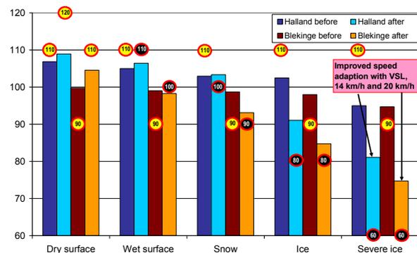
Figure: Average speeds at Hökaslätt in Halland and Bräkne-Hoby in Blekinge (both directions) at different road surface conditions with and without VSL
