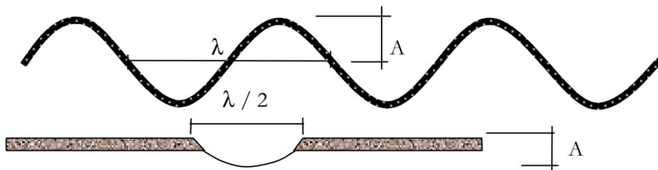
**Figure 2** Wave length ( $\lambda$ ) and amplitude (A). Above at a corrugation, below at a pothole.
