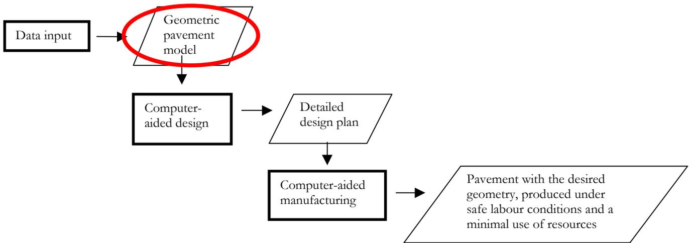
**Figure 1** The SNRA's "Procedure at road repairs "
