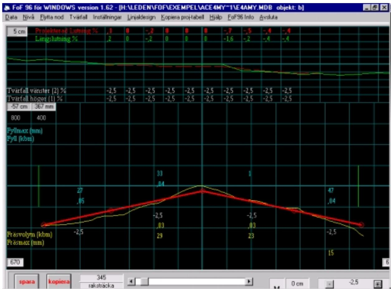
Figure 3 Geometric pavement model (green and yellow thin solid line), excluding the road environment video, used in the CAD environment. Above is the roughness profile, below the cross-section. The dotted and thick red lines show the milling as designed.
